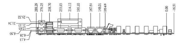
Figure 10. SDS2 Server Board Rear I/O Panel
